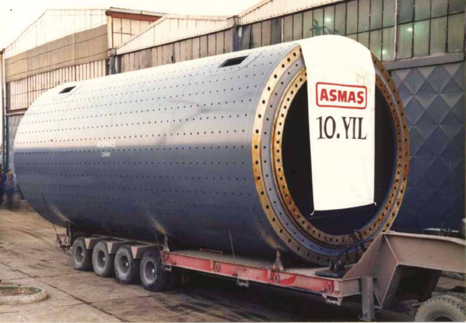
Batı Anadolu Cement Company - Turkey 220t/h Cement Mill Manufacturing: ASMAŞ
